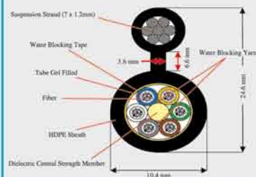
Duct Uni-Tube (Non-Metallic) Central Buffer Tube Type Cable
